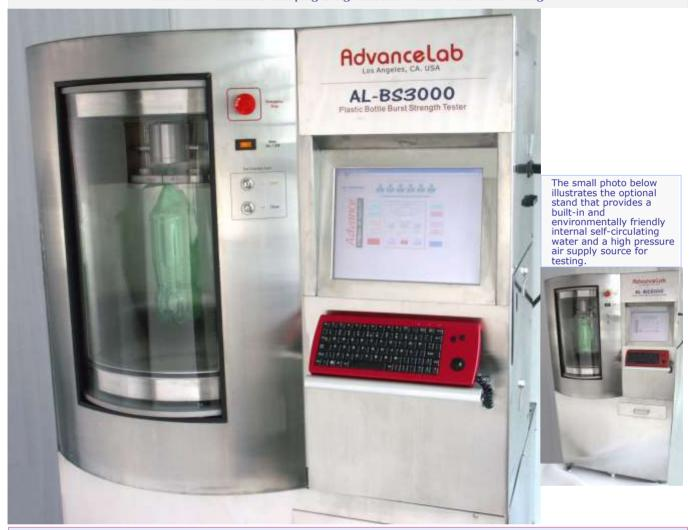
Optional environmentally friendly, internal and integrated self-circulating water and high pressure air supply source eliminates the need for a cumbersome external liquid nitrogen supply
